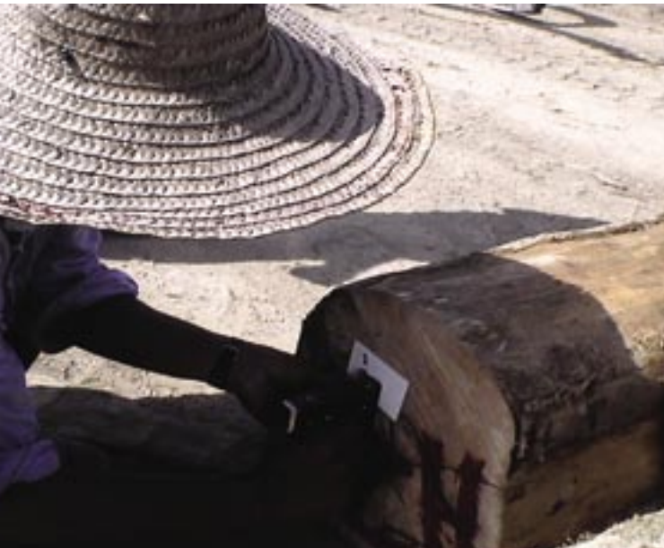
A worker implanting RFID tag
